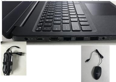
3. Plug the USB printer cable into the USB port on the right side of the laptop. The other end of the USB Printer cable plugs into the printer. It will only fit one way.
