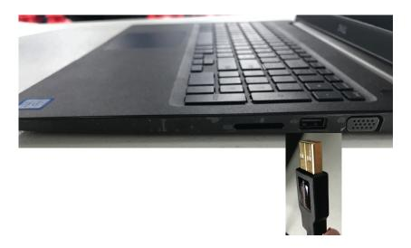
4. Plug in the USB cable to the printer. Plug the printer into the yellow extension core and turn on the printer.
